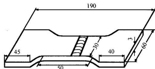
Fig. 1 Geometrical characteristics
